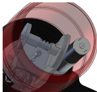
Wire supply rotates along with head
