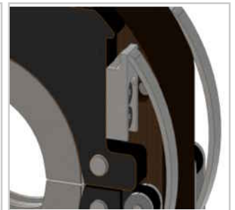
Adjustable spring- loaded system: to account for tube "out of round"
