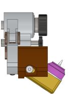
Torch angle adjustment: welding under flange or short T angle
