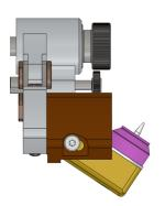
Torch angle adjustment: welding under flange or short T angle
