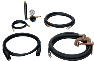
Cart Accessory Kit 301528 Single-wire feeder kit for use with running gear 301523. See note below for dual-wire feeder kit. Consists of flowmeter regulator with 5-foot (1.5 m) gas hose, 10-foot (3 m) 4/0 feeder weld cable with lugs, 15-foot (4.6 m) work cable with 600-amp C-clamp, and 9-foot (2.7 m) ArcConnect control/motor cable. Dual kit comes with an additional flowmeter regulator and gas hose.
