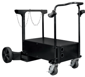
Deltaweld 350/500 Running Gear 301523 Features small footprint, dual-cylinder rack, chains for gas cylinders, ergonomic handle design and lockable front casters with two torch holders, and storage area below.
