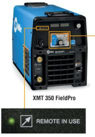
**Remote in use indicator** provides convenient feedback indicating an ArcReach<sup>®</sup> wire feeder is controlling the power source. While under ArcReach control, process and voltage/ amperage adjustments are locked out, preventing accidental changes by personnel other than the welding operator.
